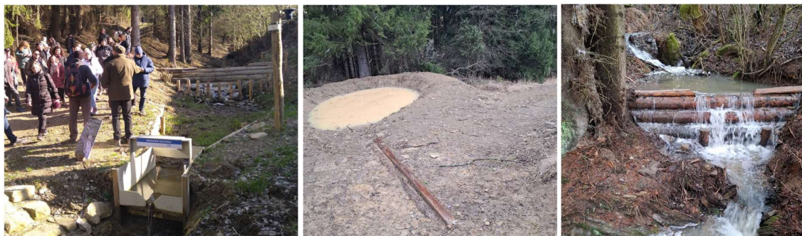
Monitoring facility for observing flows, precipitation, and water retention facilities filled with collected rainwater during heavy rainfall
